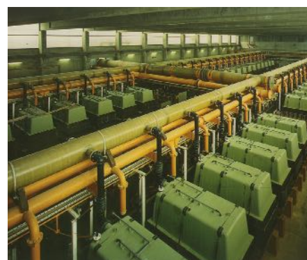
Chloralkali electrolysis yields chlorine, hydrogen and sodium hydroxide (photo: Lurgi)
